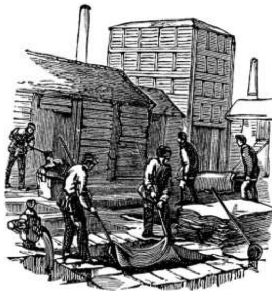
Fig. 9. Moving hides from one vat to another. Vats contained lime solutions, bate, or tanning solutions.
